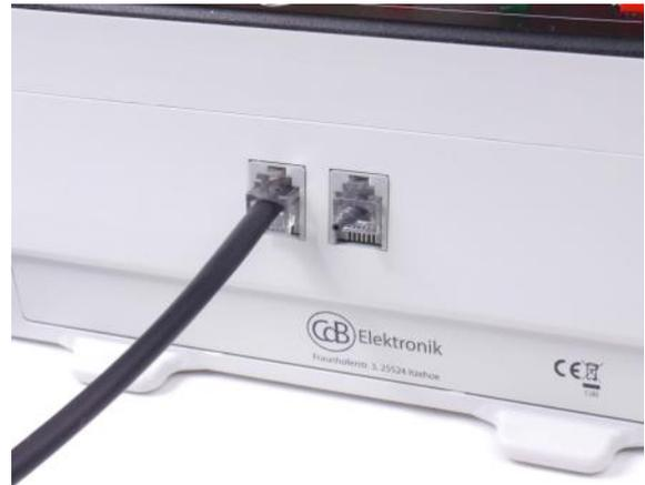
If several CAN-StellPults are to be connected together, the terminal resistor can also be removed in order to free the jack for connection to the other CAN-StellPult because one remaining resistor in one CAN-StellPult suffices for the whole composition of CAN-StellPults.
