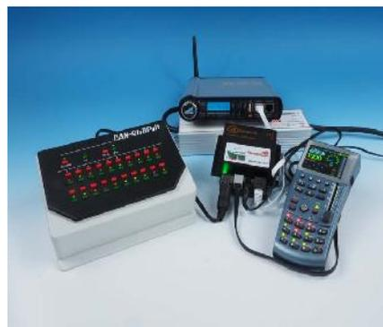
If you even need several CAN-StellPults at one desk, you can also connect devices directly to each other using the two jacks on the back. A suitable cable is also available for this purpose.
